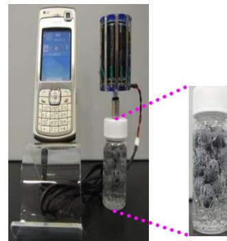
A cellular phone recharged from a 2W PEMFC powered by H<sub>2</sub> produced from catalyzed hydrolysis of NaBH<sub>4</sub> over light-weighted Co catalyst
