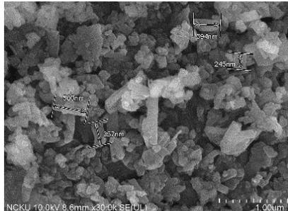
Zeolite CAN prepared from diatomite
