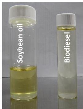
Biodiesel made from catalyzed transesterification of soybean oil in methanol over zeolite catalysts
