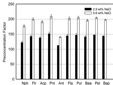
Performance of the L<sub>3</sub>-phase extraction on trace hydrophobic solutes such as polycyclic aromatic hydrocarbons (PAHs).
