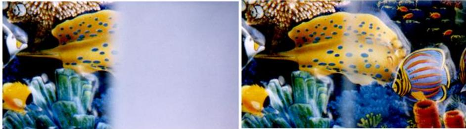
Liquid crystals can be used for LC display. Voltage bias changes LCD from "OFF" state to "ON" state. The response time could be really fast.
